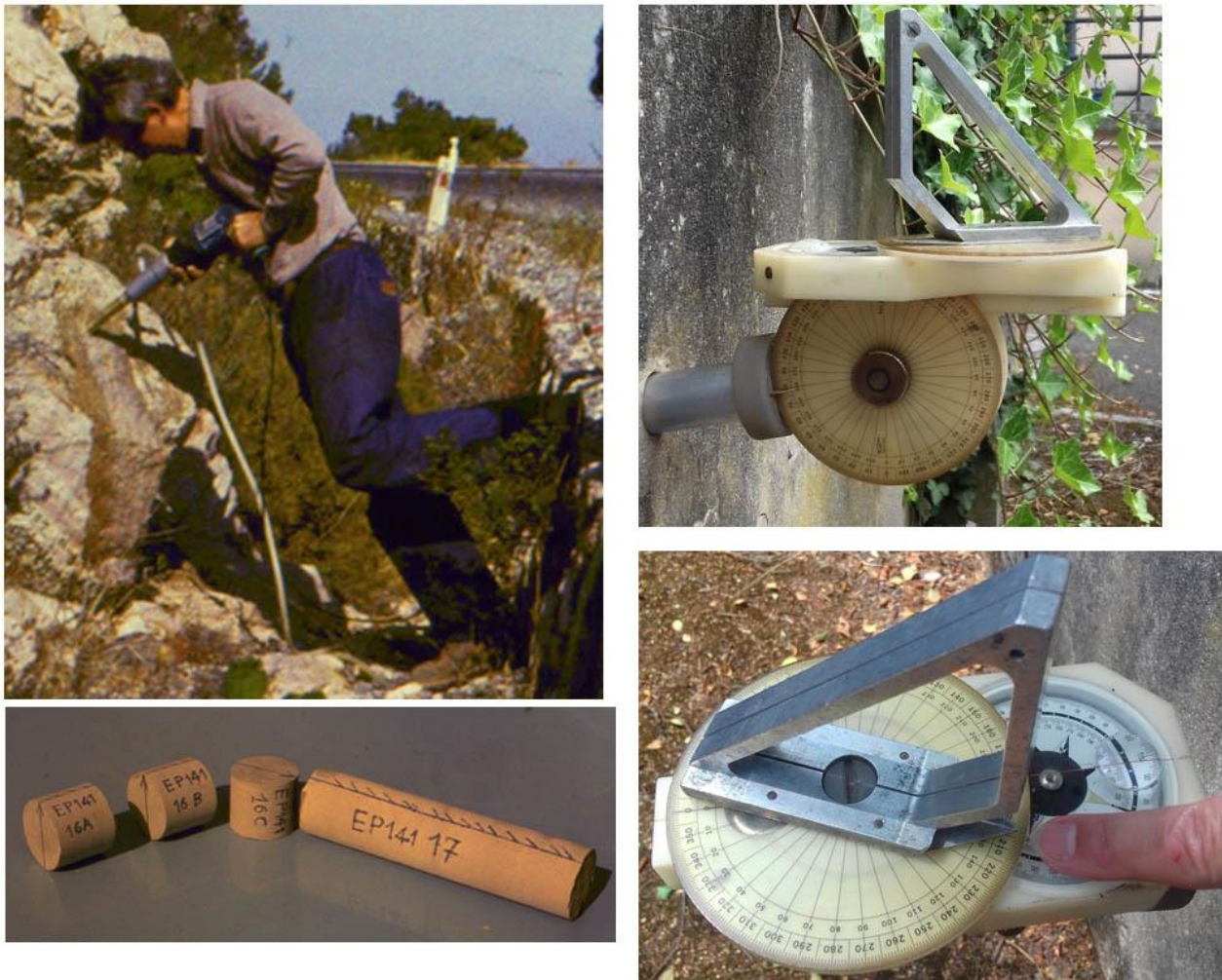
Figure 12: Paleomagnetic sampling and orientation
