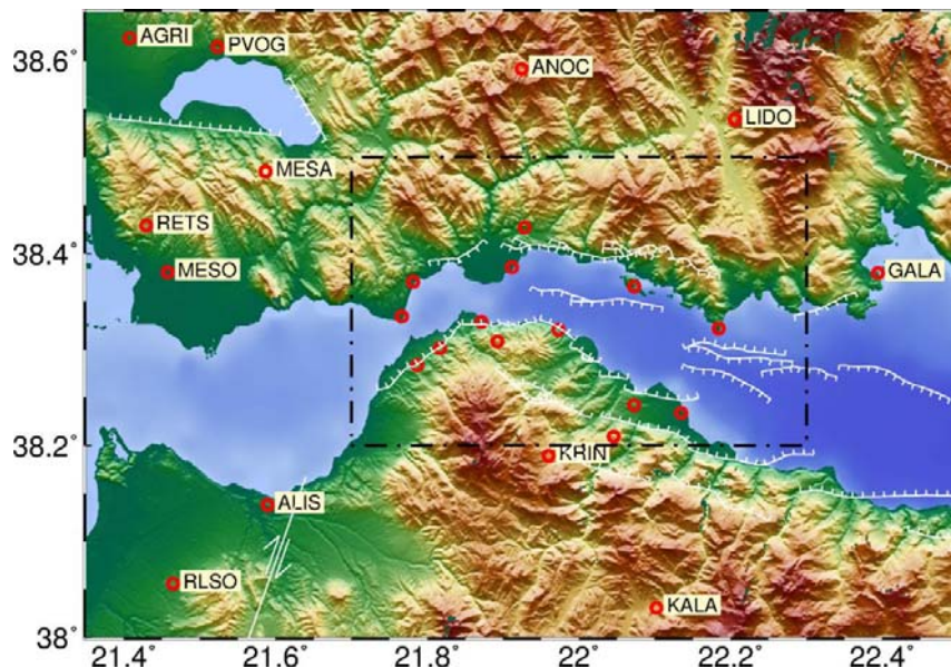
Figure 3. The stations shown are the GNSS ones (see http://crlab.eu for all maps). The seismic stations have a similar repartition. The small rectangle represents the “core area” where a higher density of sensors is concentrated. Although less numerous, the wide area is crucial to constrain both deformation and seismicity of the rift at the broad scale.
