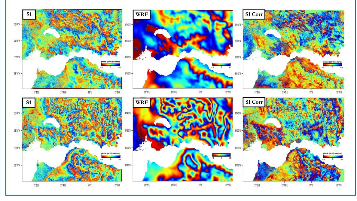
terrestrial dataset (ASTER 1s global GDEM v2) is introduced. Model output is recorded every 30 minutes, from which Zenith Hydrostatic Delays (ZHDs) and Zenith Wet Delays (ZWDs) are calculated.
