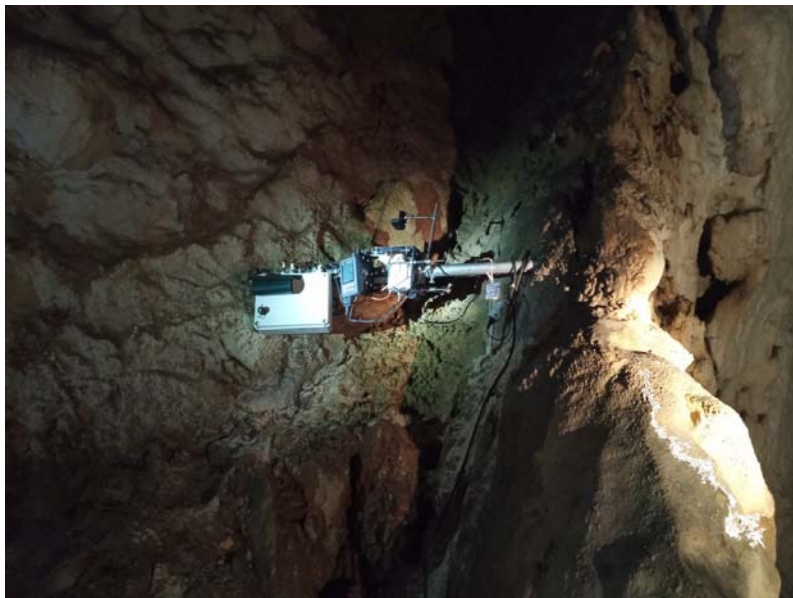
Figure 4. Field trip at the Postojna cave : strainmeter in a fault
