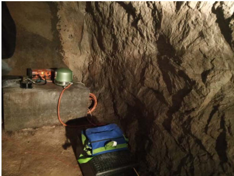
Figure 3. Field trip at the Postojna cave : seismometer and strong motion instruments
